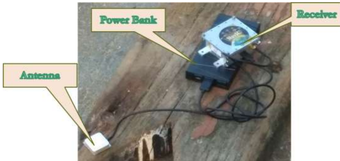
Figure-3: NavIC Messaging and Positioning Receiver Setup with power bank and Antenna
